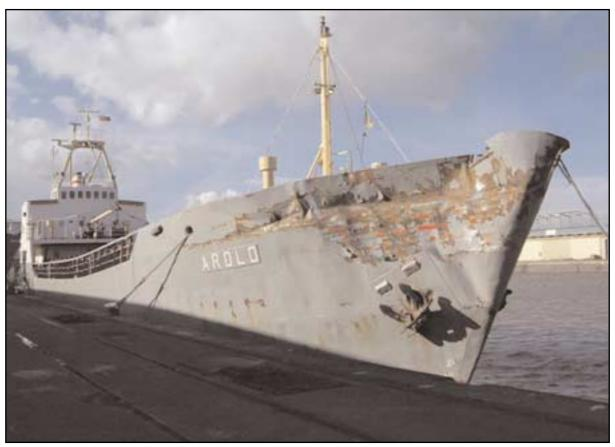
Arold berthed at King George Dock, Hull, showing damage to starboard bow
